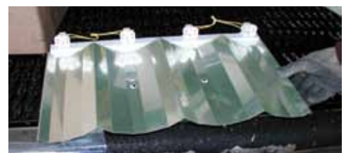
A closer look at the mirrored reflector that can double or triple the lumen output of a lamp.
