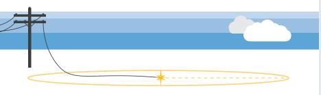
Downed power lines can energize the ground up to 35 feet away — so keep your distance.
